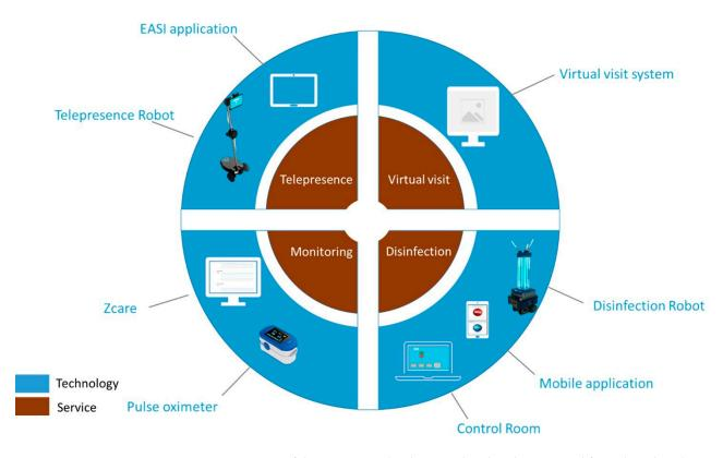
**Figure 2.** Overview of the assistive technology used within the proposed fast pilot. The telepresence service was performed with the robot and with the tablet. As for the telepresence service with the robot, two telepresence robots were used: Ohmni and Double robot.
