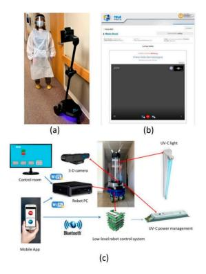
Figure 3. (a) Ohmni robot and professional caregiver during the telepresence service in a residential facility; (b) user interface developed for the virtual visit service; (c) disinfection robot and its main components.
